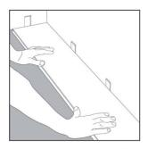
Step 1: Begin installation from left to right. Insert spacers at the ends where planks meet the wall to maintain an 8mm expansion gap.
